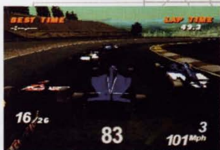
F1 copes easily with several cars on-screen at the same time without stepping down to 'chug' mode. Cars in the distance use less graphical detail, but the effect isn't obvious to the player
